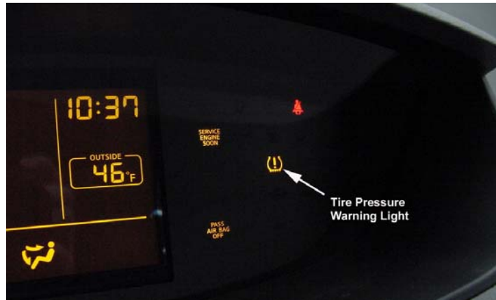
Picture 6: Low Pressure Warning Light Shown Illuminated
