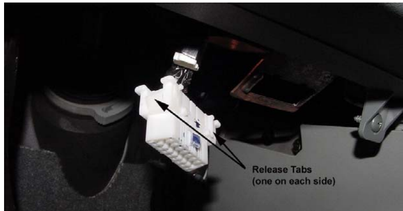
Picture 2: Release tabs on DLC.
