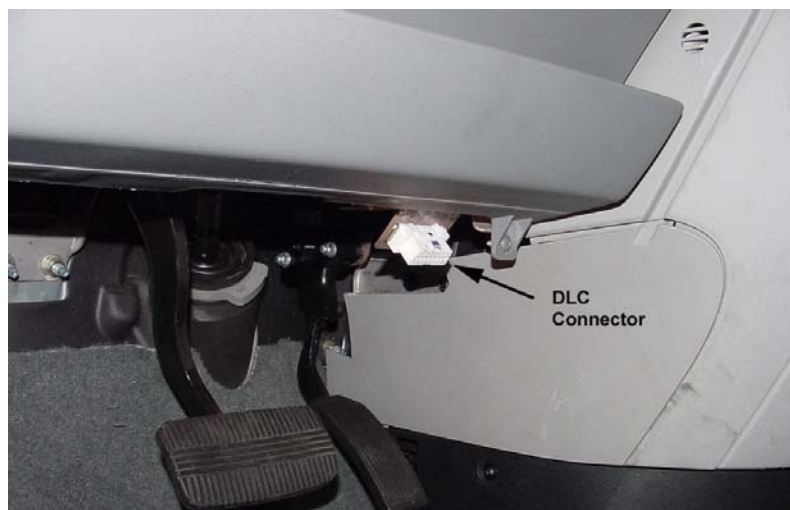
Picture 5: DLC Connector shown under dash.
