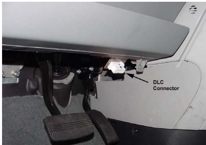
Picture 1: DLC Connector shown in under-dash location.
